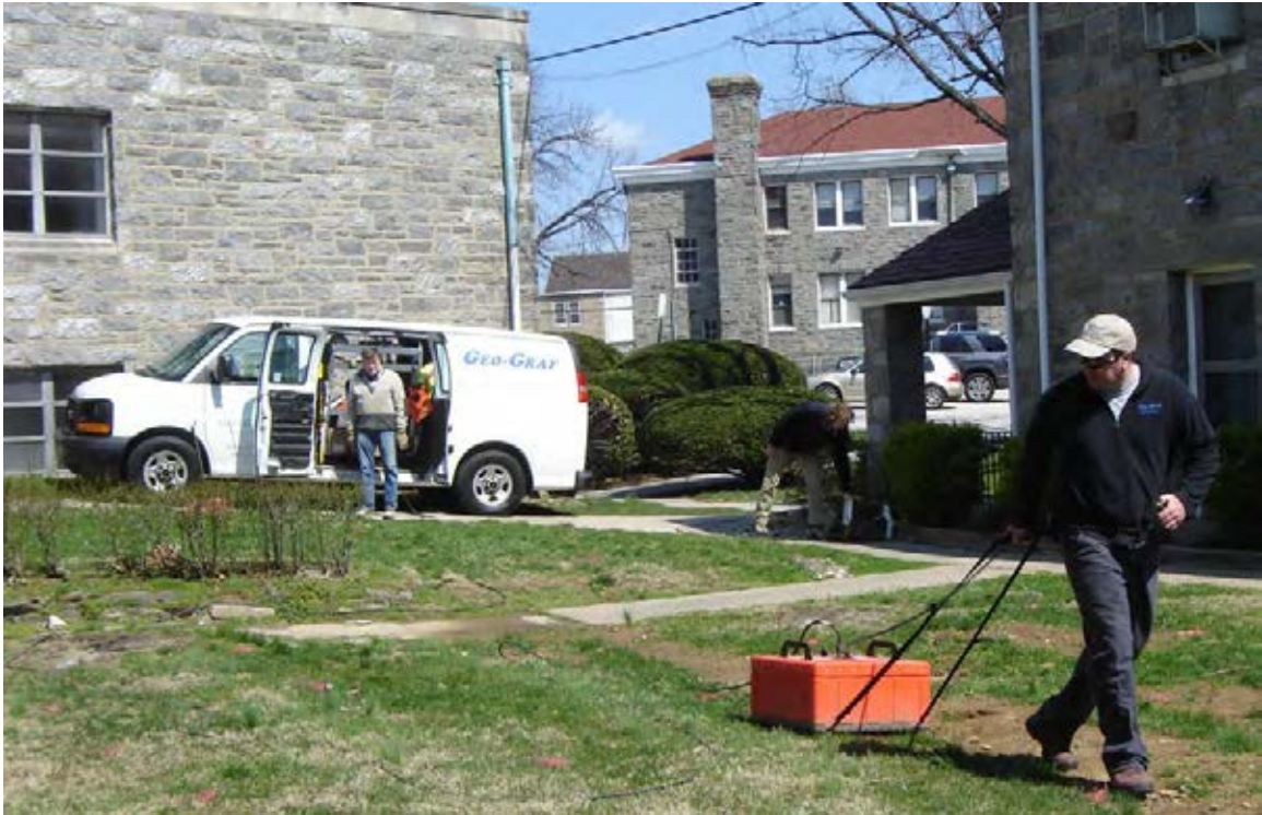
Figure 1 Mr. Graf, from Geo-Graf Incorporated, conducting the Ground Penetrating Radar.
