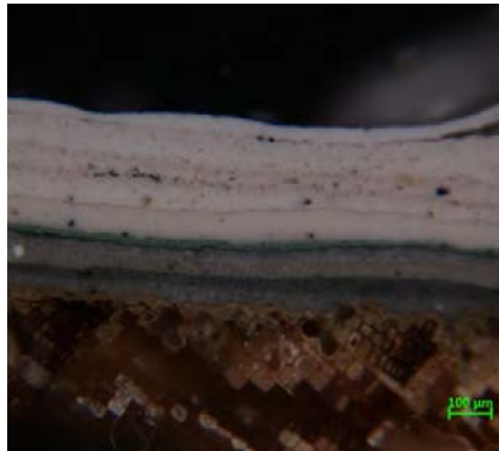
Figure 7 Sample from exterior window on north facade, 2010. layer following the yellow paint campaign.
